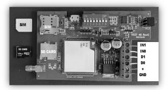
Inside the unit there is a terminal block for connecting the unit to the controller, a dipswitch for setting up the unit, a SIM card tray, and a SD card tray.
